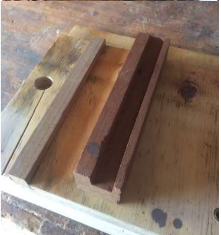
Long edge jointing jig showing end stop removed for surface planing
